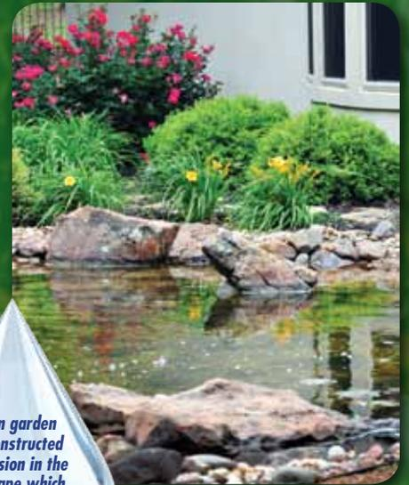
*A rain garden is a constructed depression in the landscape which collects runoff and allows water to percolate into aquifers within 24 hours.*
